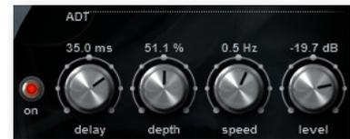
The **Delay** knob specifies in milliseconds, the delay between the original signal and the secondary signal. A delay of around 40 ms is typical, so is often a good starting point when crafting a specific effect.
