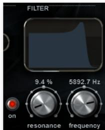
The Frequency knob determines where the sound starts to be filtered out. The Resonance knob specifies how much the filter “rings” at the dialed frequency. The higher the resonance knob is set, the more focused this ringing becomes.
